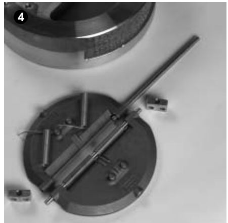
Remove support plates, cover springs and withdraw hinge pins.
