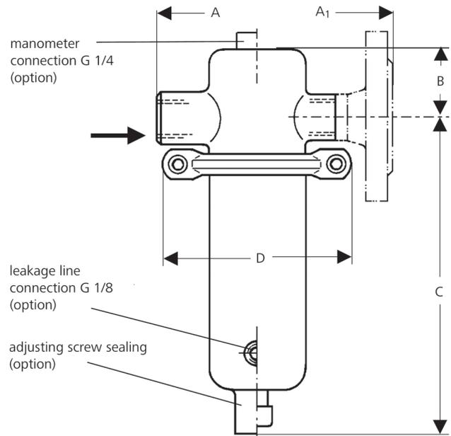
\*overall length tolerances in acc. with DIN EN 558
