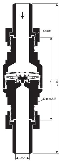
Design with union butt-weld nipples
