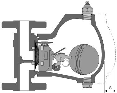
To remove the cover a withdrawal space S of 240 mm is required.
