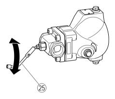
You can check the correct functioning of the equipment during operation using the GESTRA ultrasonic measuring unit VAPOPHONE<sup>®</sup> or TRAPTEST<sup>®</sup> (VKP 40 and VKP 40plus).
