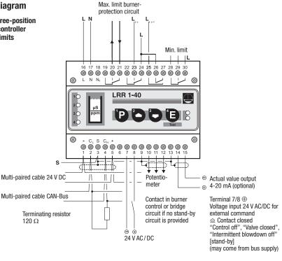
Two- or three-position stepping controller with one limit value and intermittent blowdown function
